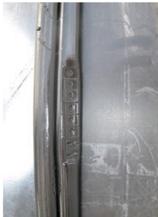
Fig. 14: Welding bead with stamp mark (Arabic series of numbers)
