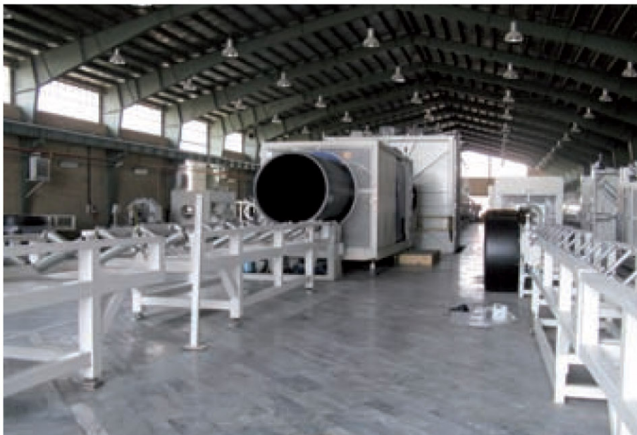
Fig. 3: Production plant in Saveh with extrusion line for large-dimension PE pipes
