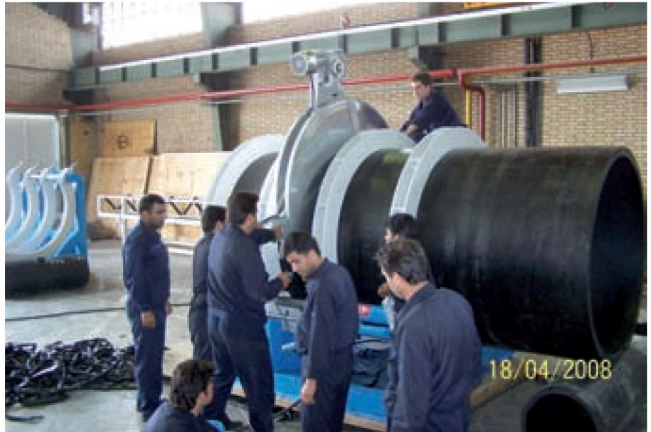
Fig. 6: Welders during training course with CNC welding machine for the welding of large-dimension pipes
