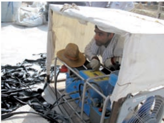
Fig. 8: Welder and CNC-control unit of the welding machine with sun protection and air conditioning by means of a ventilator
