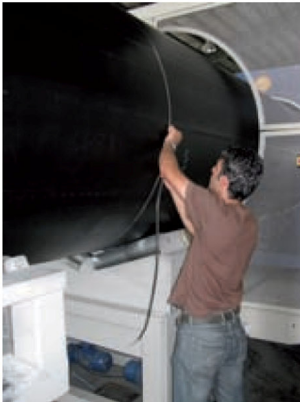
Fig. 5: A staff member of P.E.S. Co. examining the outer pipe diameter with a circometer
